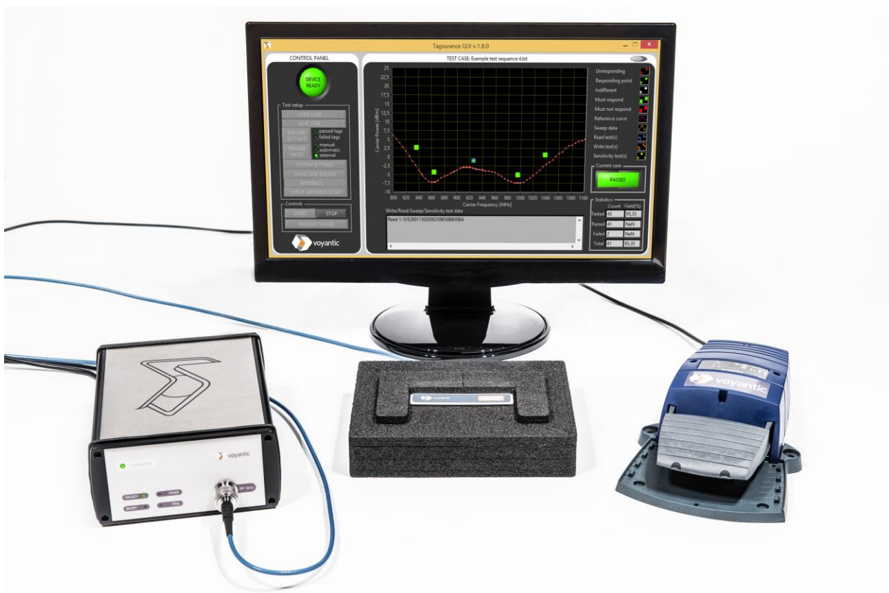
Fig 2 Basic measurement setup with Manual Test Station Kit
